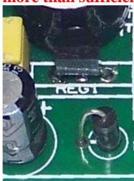
**The regulator flat face should be facing the diode and capacitor.**
